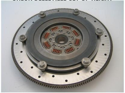
With the disc installed on the flywheel and the pressure plate in place, check the diaphragm "Belleville" spring set for correct set up height.
