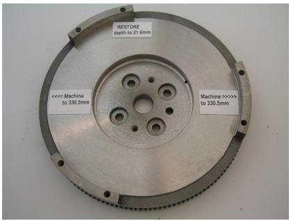
As shown above, the cover mounting surface of the flywheel must be increased to accommodate the larger clutch.
