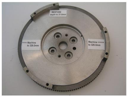
As shown above, the cover mounting surface of the flywheel must be increased to accommodate the larger clutch.
