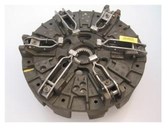
229 2802 FE = 88mm bolt fixing height, the assembly spigots on the outside of the cover and the flywheel has no step (completely flat)
