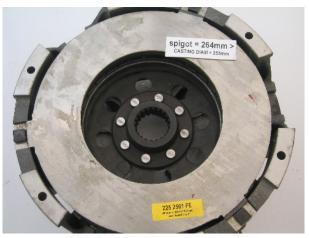
225 2501 FE = 250mm internal base plate diameter, the assembly spigots on the inside of the cover, the flywheel has a 2.0mm step (positive).
