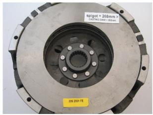
226 2501 FE = 260mm internal base plate diameter, the assembly spigots on the outside of the cover and the flywheel has no step (completely flat)
