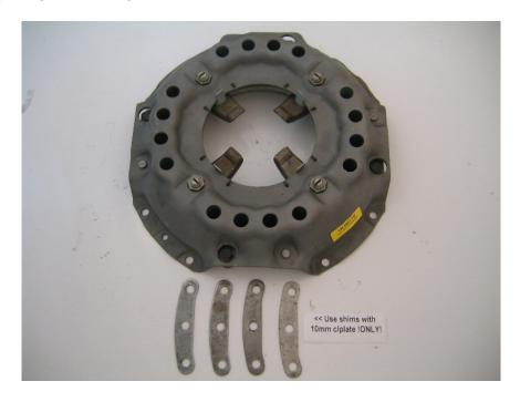
Check clutch plate thickness prior to installation.
