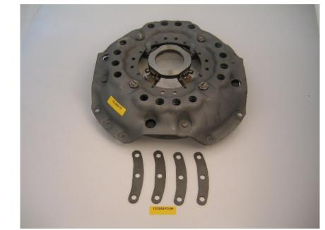
Check clutch plate thickness prior to installation.
