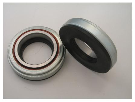
The part number above includes a special plastic sleeve, this is pressed into the bearing and is designed to reduce the wear and heat that would otherwise be transferred through the clutch diaphragm.
