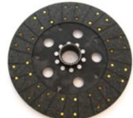
Application Commonly used across the standard tractor and industrial tractor range for example; headers, combines, backhoe loaders and crawlers in lighter applications. Also used for the PTO drive in many dual type clutch assemblies.
