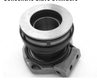
This combined hydraulic slave cylinder and thrust bearing assembly is designed to operate directly in front on the clutch cover assembly. The unique design eliminates the need for complex and sometimes expensive clutch release fork and linkage mechanisms.
