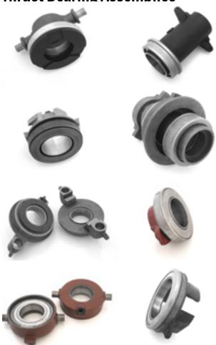
In dual applications the main and PTO thrust bearings can often be incorporated into a single carrier assembly with one operating inside the other. The bearings are press on type which can be replaced if the carrier is serviceable.
